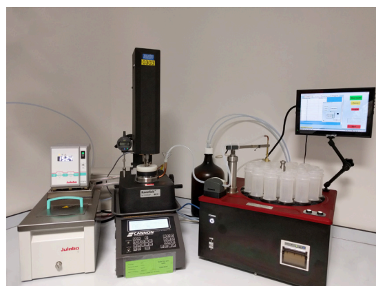
Ravenfield® BS/C+ HTHS Viscometer shown with Model DR Autosampler and temperature controlled bath
